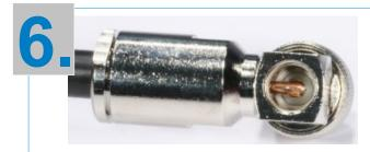
Slide the prepared cable end into the connector housing until stop. Tighten smoothly with two wrenches 17 mm and 18 mm so that there is still a small gap visible between the nut and the connector Carefully solder the center conductor of the cable to the center contact of the connector.
