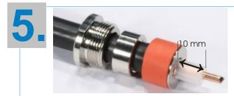
Remove foil with a knife. Trim the dielectric to a length of 10 mm.
