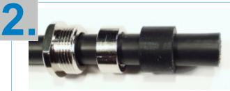
Slip the nut, the pressure ring and the rubber gasket over the cable end. Hint: With a small amount of vaseline the rubber gasket will slide more easily.
