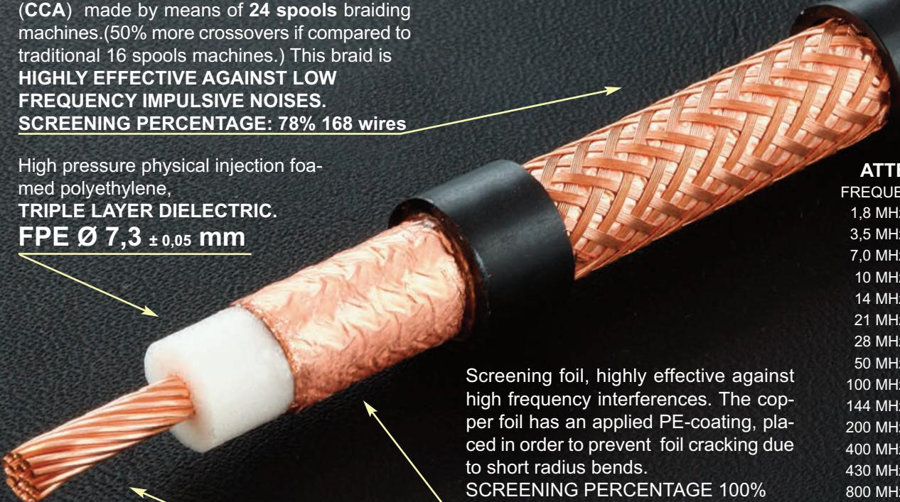
Screening foil, highly effective against high frequency interferences. The copper foil has an applied PE-coating, placed in order to prevent foil cracking due to short radius bends.
