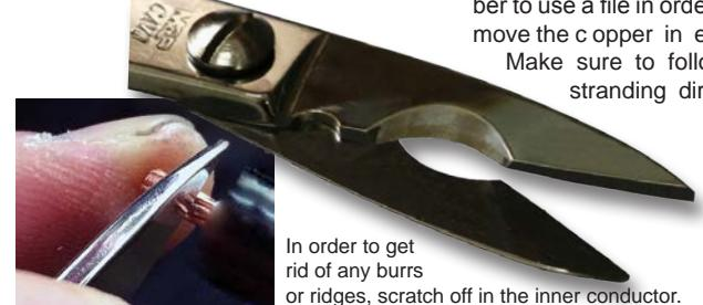
In order to get rid of any burrs or ridges, scratch off in the inner conductor.
