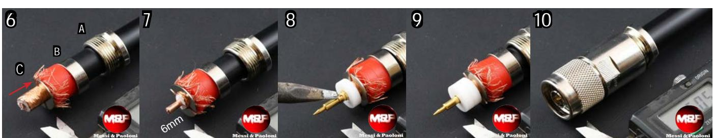
Push component C between the foil and the braid until it stops against the red PE jacket.
