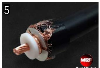
Insert the first teflon disc like in the above picture.
