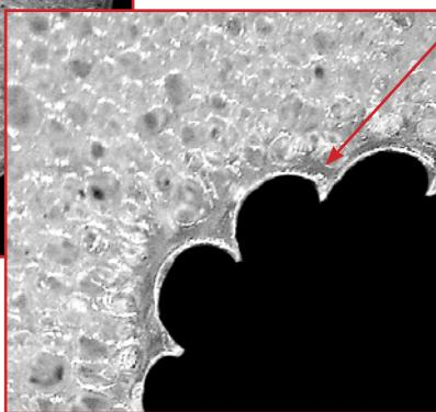
In the image at your left, we can clearly distinguish at 150 x magnifications, the mechanical structure of the **Gas Expanded TL (triple layer)** technology.
