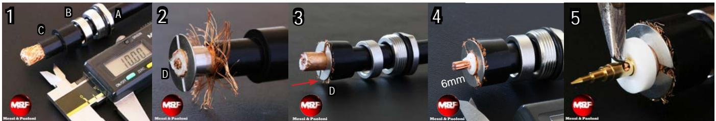
Insert in the cable components A, B, C and immediately after, make a circular cut on the black PVC jacket at the indicated length shown in the caliber (in mm). Subsequently remove it.
