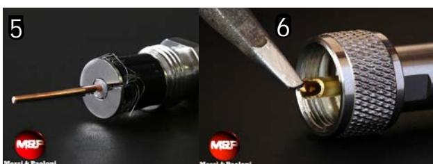
Cut and remove the tape and dielectric for a lenght as shown in the picture.
