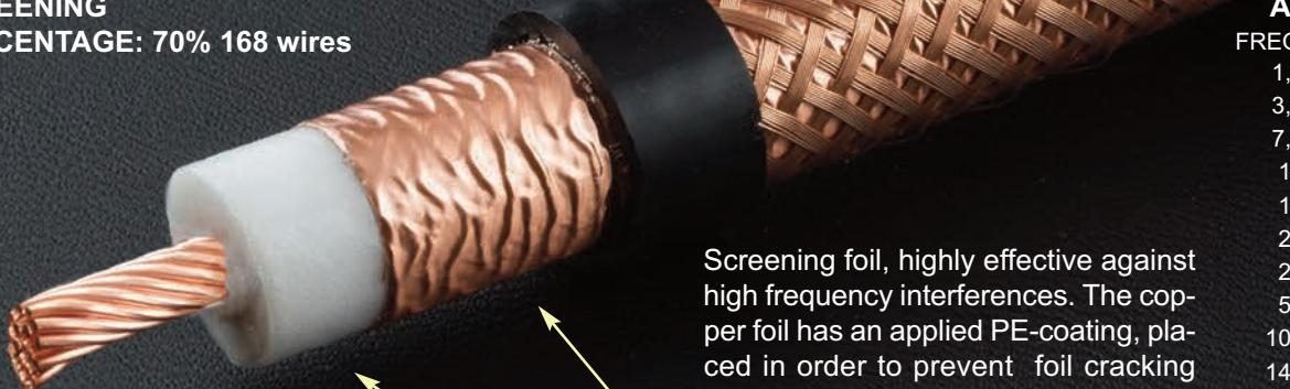
Inner conductor made of 19x0,78 stranded, geometric and concentric annealed copper wires. Purity 99,99%. (annealed = thermal softening process) **(19x0,30 inches)**
