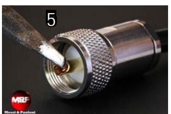
Fasten together the connector and component A, until it will be pressed against the connector body. Inside, the rubber component C (pic 1) will expand, granting optimal sealing against moisture and a perfect contact to ground.
