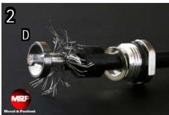
After having made the first cut, as shown in picture 2, rotate the cable 180 degrees and make a second cut in the same way, in order to facilitate the introduction of component D (pic.4 and 5)
