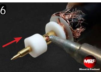
Insert the second teflon disc like in the above picture and subsequently the central pin. Solder the pin to the inner conductor, inserting tin in the provided hole. Avoid heating the pin for a too long time in order not to damage with excessive heat the cable dielectric (which is not made in teflon!).
