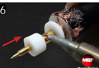
Insert the second teflon disc like in the above picture and subsequently the central pin. Solder the pin to the inner conductor, inserting tin in the provided hole. Avoid heating the pin for a too long time in order not to damage with excessive heat the cable dielectric (which is not made in teflon!).
