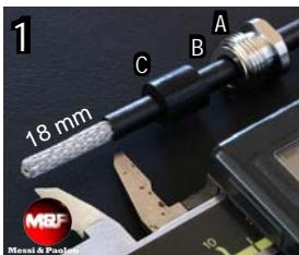
Insert in the cable components A, B, C and immediately after, make a circular cut on the jacket at the indicated length shown in the caliber. (in mm). Subsequently remove it.
