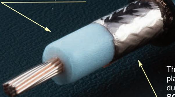
The copper foil has an applied PE-coating, placed in order to prevent foil cracking due to short radius bends.
