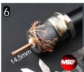
Cut and remove the tape and dielectric for a length as shown in the picture.
