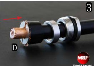
Flatten the wires as shown in the picture and cut the excess.
