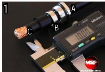
Insert in the cable components A, B, C and immediately after, make a circular cut on the black PVC jacket at the indicated length shown in the caliber (in mm). Subsequently remove it.
