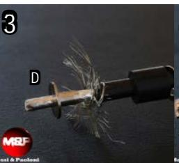
Insert component D after having opened the braid as shown in the picture.
