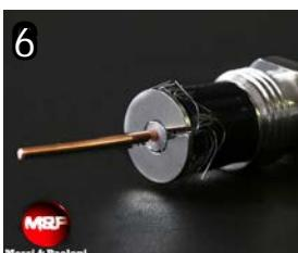
Cut and remove the tape and dielectric for a lenght as shown in the picture.
