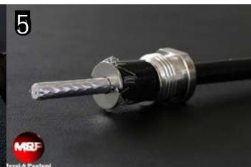
Flatten the wires as shown in the picture and cut the excess.
