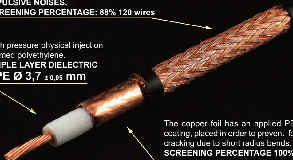
Inner conductor made of 19X0,29 stranded geometric and concentric copper wires. Purity 99,99% annealed.
