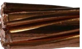
Common scissors: remember to use a file in order to remove the copper in excess. Make sure to follow the stranding direction.
