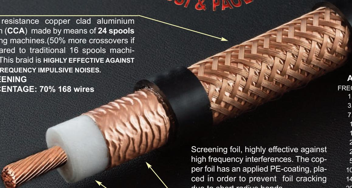
Inner conductor made of 37x0,56 stranded, geometric and concentric annealed copper wires. Purity 99,99%. (annealed = thermal softening process) **(37x0,022 inches)**
