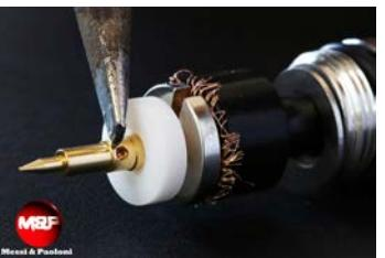
Insert in the cable components A, B, C and immediately after, make a circular cut on the jacket at the indicated length shown in the caliber. (in mm) Subsequently remove it.
