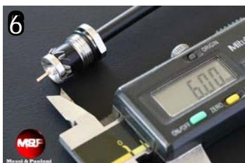
Cut and remove the tape and dielectric for a lenght as shown in the picture (in mm).
