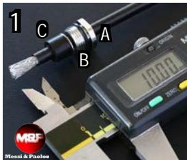
Make a circular cut on the black PVC outer jacket at the indicated length shown in the caliber (in mm). Subsequently remove it.
