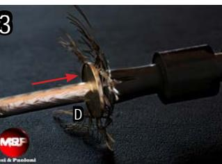
Push component D between the foil and the braid until it stops against the jacket.
