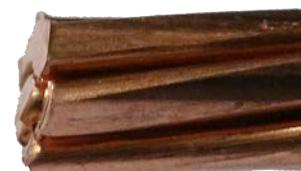
Cut made with special M&P scissors.
