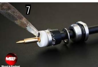
Insert one of the two teflon discs and subsequently the central pin. Solder the pin to the inner conductor, inserting tin in the provided hole. Avoid heating the pin for a too long time in order not to damage the cable dielectric. (which is not made in teflon!)
