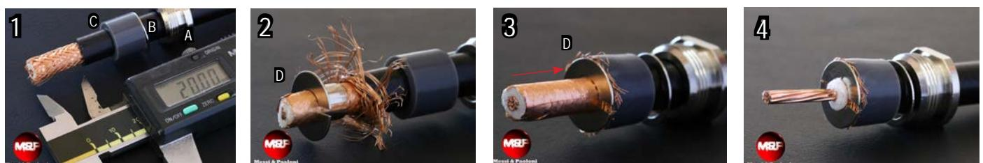
Insert in the cable components A, B, C and immediately after, make a circular cut on the black PVC jacket at the indicated length shown in the caliber (in mm). Subsequently remove it.
