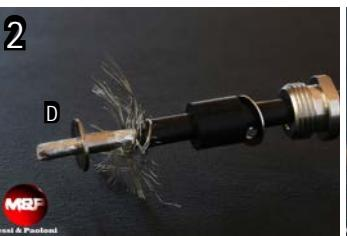
Insert component D after having opened the braid as shown in the picture.
