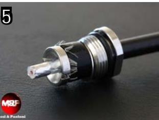
Flatten the wires as shown in the picture and cut the excess.
