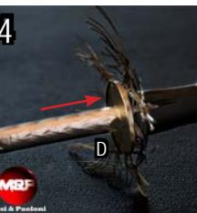
Push component D between the foil and the braid until it stops against the jacket.
