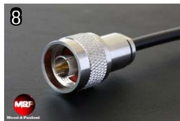
Insert the connector and fasten accurately until the o-ring present in component A, will be pressed against the connector body. Inside, the rubber component C (pic. 1) will expand, granting optimal sealing against moisture and a perfect contact to ground.
