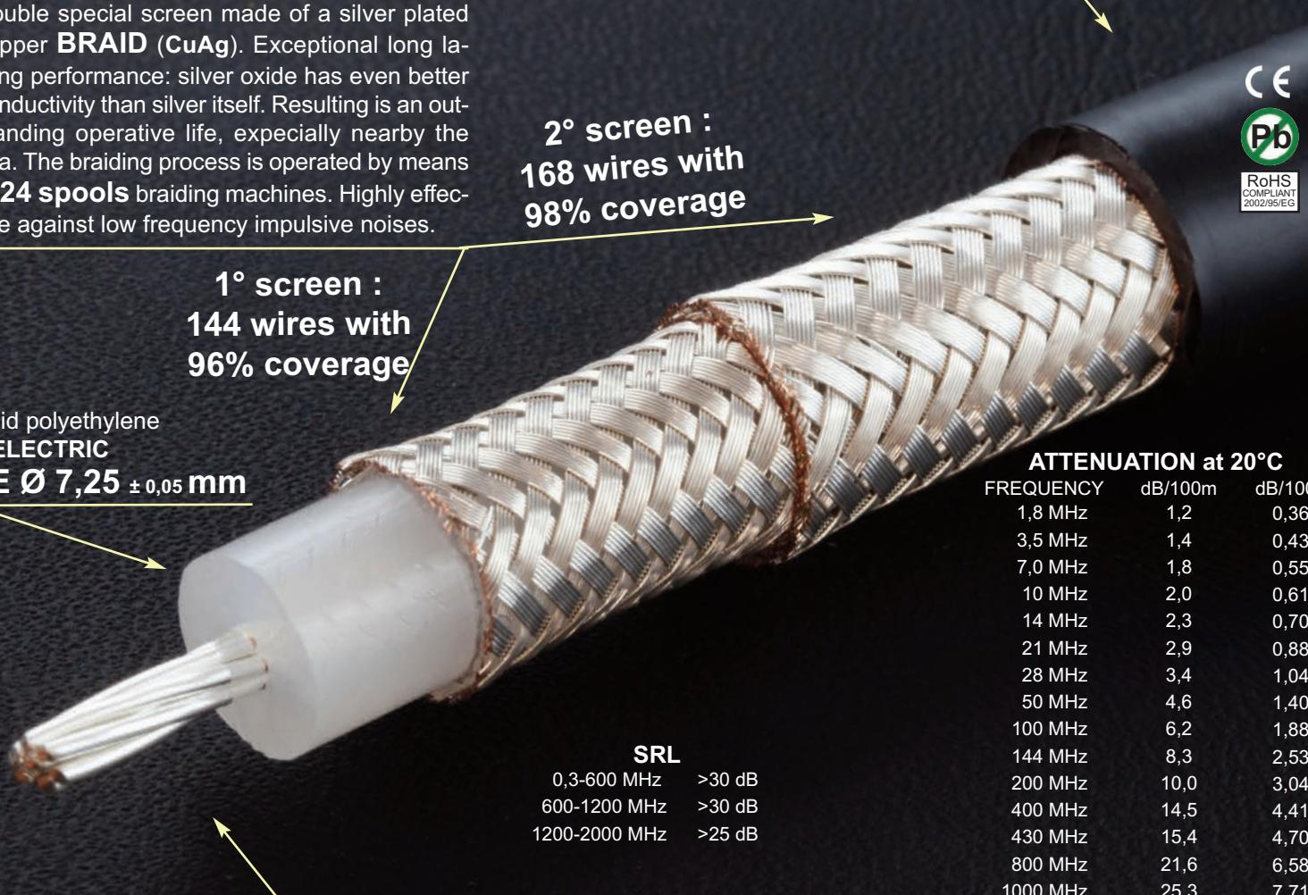
Inner conductor made of 7X0,75 stranded geometric and concentric silver plated copper wires.
