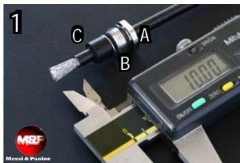
Make a circular cut on the black PVC outer jacket at the indicated length shown in the caliber (in mm). Subsequently remove it.
