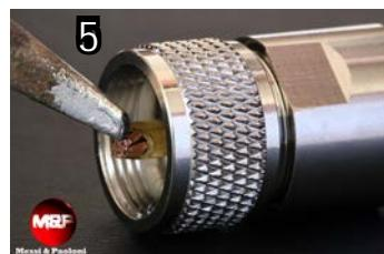
Insert the connector and solder it with tin to the inner conductor (see picture above). Avoid heating the pin for a too long time in order not to transfer excessive heat to the highly conductive copper underneath. Excessive heat deforms the dielectric which is made of foam PE and not in teflon!.
