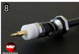
Insert the second teflon disc as shown in the picture.
