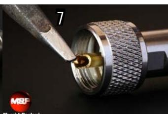
Insert the connector and solder it with tin to the inner conductor (see picture above). Avoid heating for a too long time in order not to damage the cable dielectric (which is not made in teflon!).
