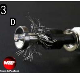
After having made the first cut, as shown in picture 2, rotate the cable 180 degrees and make a second cut in the same way, in order to facilitate the introduction of component D
