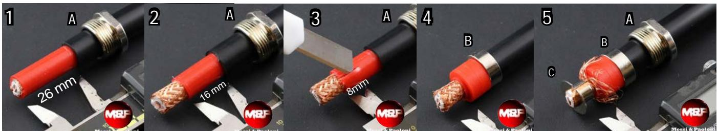
Insert in the cable components A and make a circular cut on the red PE jacket and slide it away as shown in the picture. The remaining visible red jacket must be of the length indicated by the caliber.
