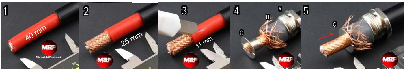
Make a circular cut on the black PVC outer jacket at the indicated length shown in the caliber (in mm). Subsequently remove it.
