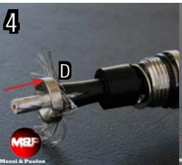
Insert component D after having opened the braid as shown in the picture. Push component D between the foil and the braid until it stops against the red PE jacket.
