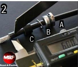
Insert in the cable components A, B, C and immediately after, make a circular cut on the red PE jacket at the indicated length shown in the caliber (in mm). Subsequently remove it.
