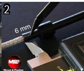
After having made the first cut, as shown in picture 2, rotate the cable 180 degrees and make a second cut in the same way, in order to facilitate the introduction of component D (pic.3 and 4)
