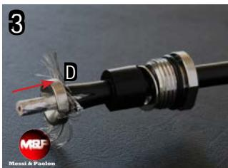
Insert component D after having opened the braid as shown in the picture. Push component D between the foil and the braid until it stops against the red PE jacket.
