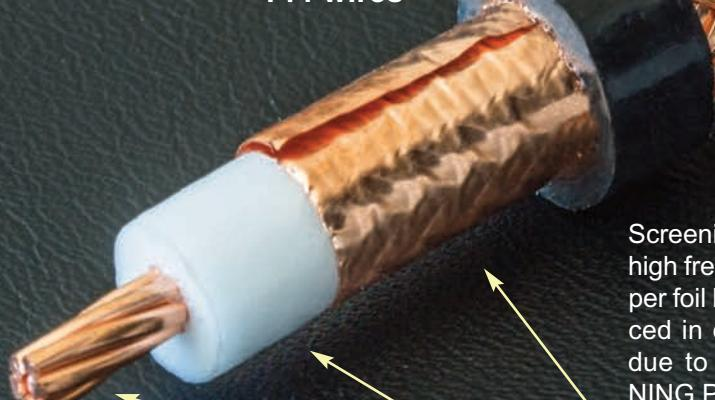
Inner conductor made of **7X1,0** stranded, geometric and concentric annealed copper wires. Purity 99,99%. (annealed = thermal softening process) (**7x0,039 inches**)
