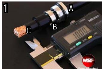
Insert in the cable components A, B, C and immediately after, make a circular cut on the black PVC jacket at the indicated length shown in the caliber (in mm). Subsequently remove it.
