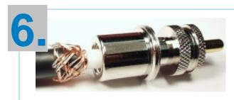
Push connector ferrule over cable end and tighten it by screwing it to stop.
