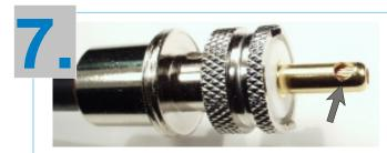
Solder center conductor carefully through the little hole..
