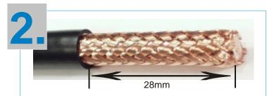
Remove 28 mm of the PVC sheath from the end of the cable with a knife.
